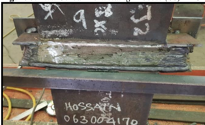
Figure 3. Flux Cored Arc Welding Process (SS) – 2G Position
