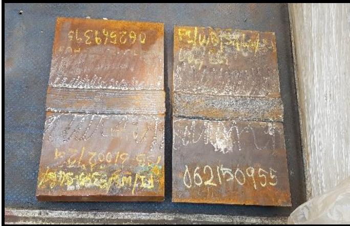
Figure 5. Test Coupon in 2G & 3G Welding with FCAW
