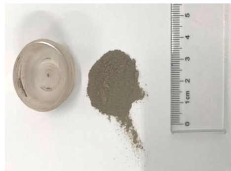
Figure 9. a) Obtained Overall Efficiencies for the Flow Rates of 11.67, 13.3 and 16.67 (l/min) b) Collected Particles by the Cyclone in the Dust Collector Chamber
