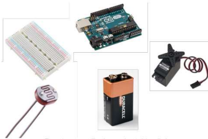
Figure 14. Most Relevant Hardware Provided to the Students (left to right): Photoresistor, Breakboard, Arduino UNO, Battery, and Servo Motor
