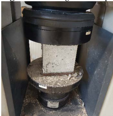
Figure 5. Testing the Compressive Strength of Concrete
