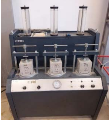
Figure 6. Testing the Depth of Water Penetration under Pressure
