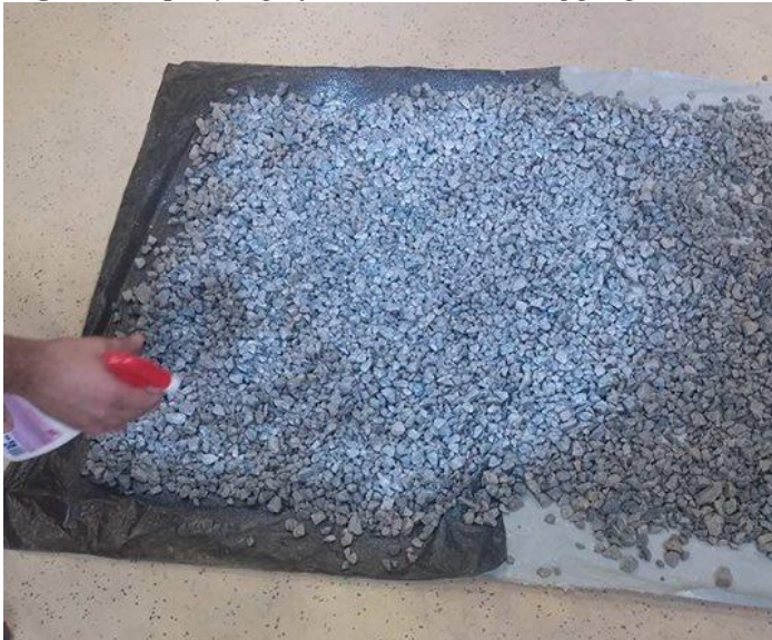
Figure 1. Spraying of Latex over the Aggregate
