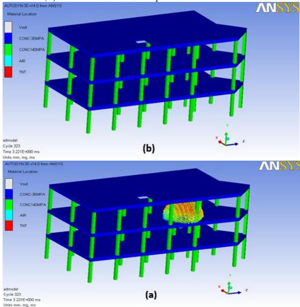
**Figure 14.** *The 1D Wedge Model Remapping at 15 ms, (a) Blast Form and (b) Concrete Erosion*
