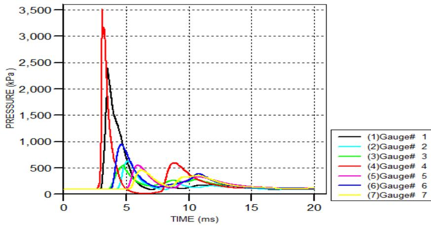
2D Box Model Remapping Results (Blast at Level 7875mm)
