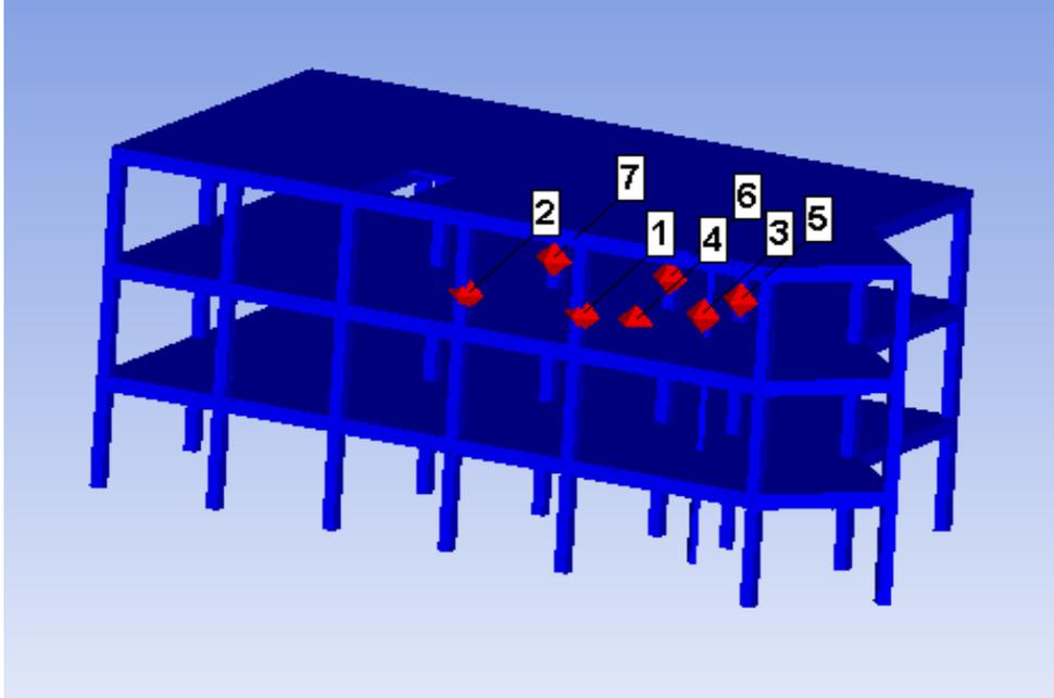
1D Wedge Model (Blast at Level 7875mm)
