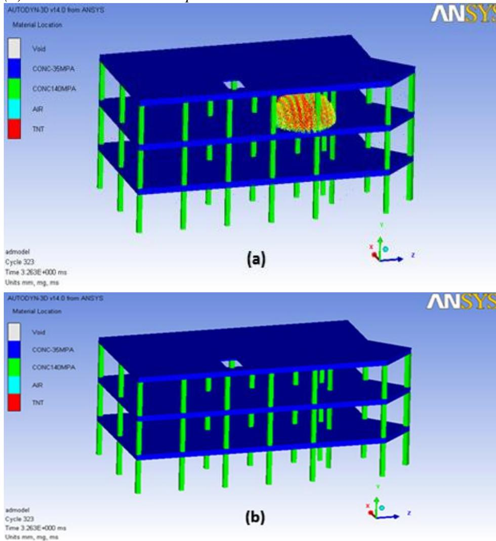
**Figure 17.** The 2D Box Model Remapping at 15 ms, (a) Blast Form and (b) Concrete Erosion
