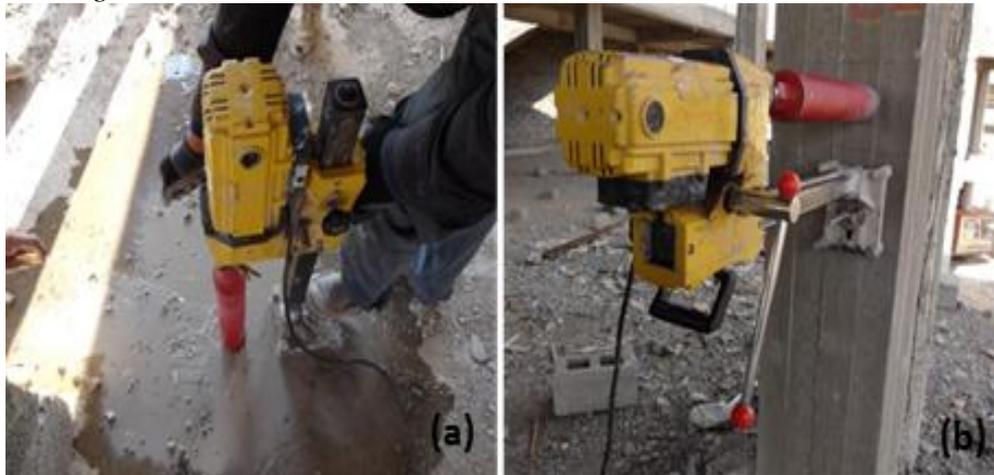
A coring bit with 75 mm in diameter was used to drill the concretes. The alignment was controlled by fixing the core machine on the floor using bolts. For ensuring compliance with the specification  $h/d \geq 1$  for cores was taken into account, as shown in Figure 5. The specimens were tested in a laboratory as shown in Figure 5. The dimensions and the density of the concrete cores have been illustrated in Table 2.
