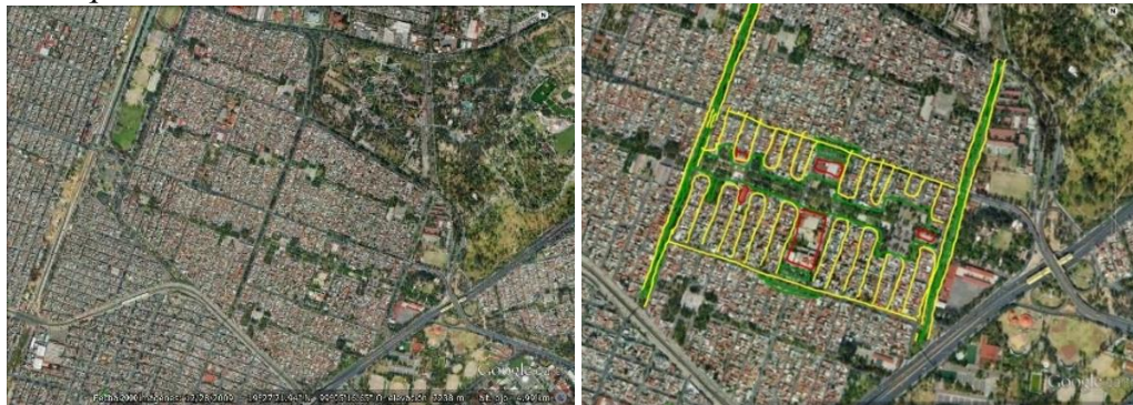
Figures 31 and 32. Aerial Views 2 Showing, on the Left, 1 st and 2 nd Sectors of the Development; on the Right, a Close-up to the Park System: Parks, Border Avenues and Squares in Green, Street Horseshoe Circuits in Yellow, and Services in Red
