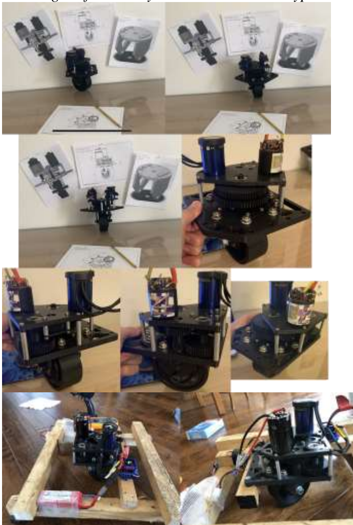
Figure 11. Several Images of the Prototype Swerve Drive Module, Along with the Images of the Dolly Swerve Drive Prototype Assembly
