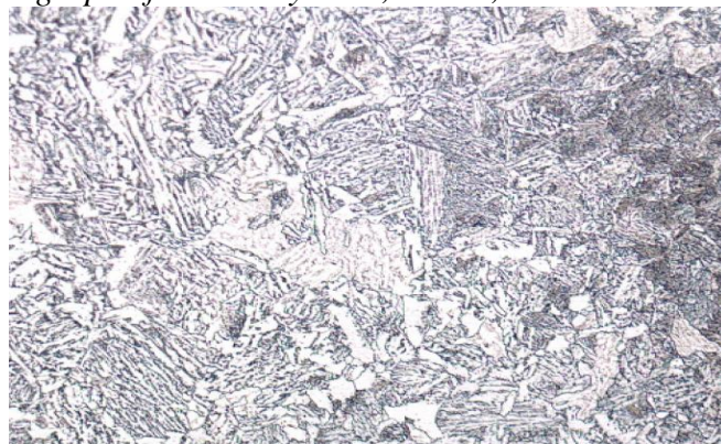
Figure 5. Micrograph of Boundary Area, etched, 500:1
