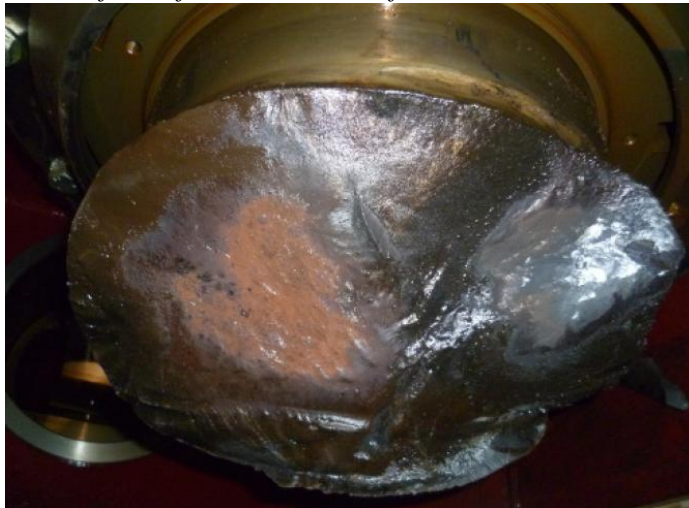
Figure 1. Crack Surface of the Broken Shaft
