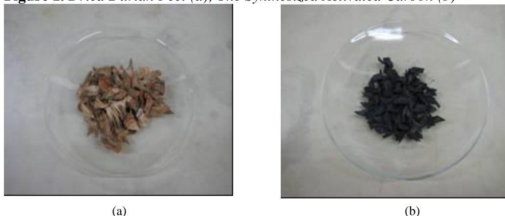
Figure 1. Dried Durian Peel (a); The Synthesized Activated Carbon (b)
