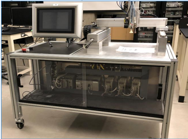
Figure 1. XYZ Gantry Table Setup
