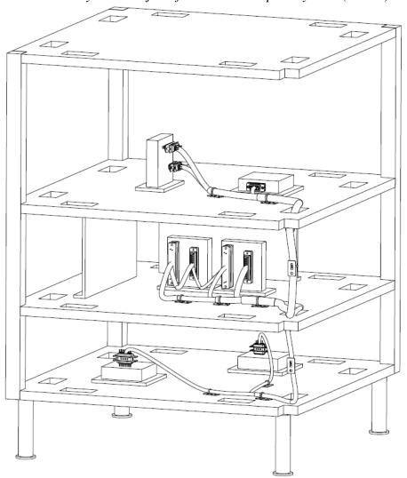
**Figure 5.** Manufacturing Drawings of the Harness Design Project of Power Subsystems (MUSE)
