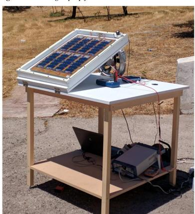
**Figure 10.** Testing Sep-up for the UPMSat-2 Solar Panels
