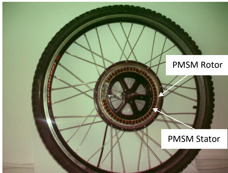
Figure 2. Photograph of the Permanent Magnet Synchronous Motor Mounted on the Bicycle Wheel (Digă, 2015)
