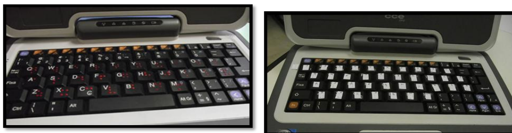
Picture 2. Customization of the educational laptop keyboard with colored glue for a student with 5% of vision and with labels in sign language for a deaf student
