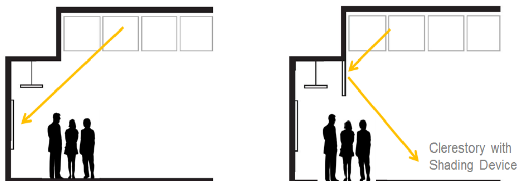
Figure 8. Shading Device to Prevent Glare on Projection Screens
