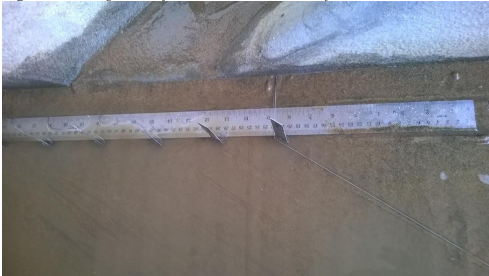
Figure 2. Arrangement of Vanes at the Entrance of Intake Canal
