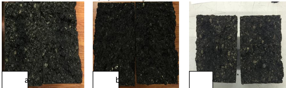
Figure 3. Investigation of Stripping of Wet Subset Samples after Testing. a) HMA; b) WMA-Evotherm; c) WMA-Sylvaroad
