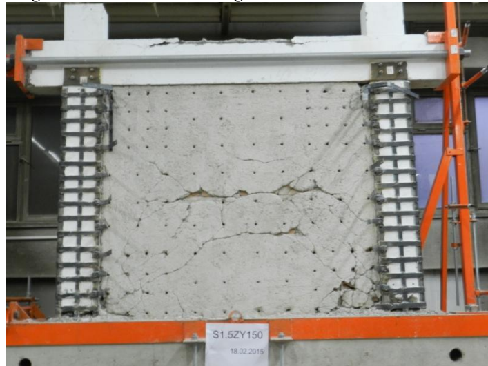
Figure 20. Diagonal Tension Cracking in the Walls
