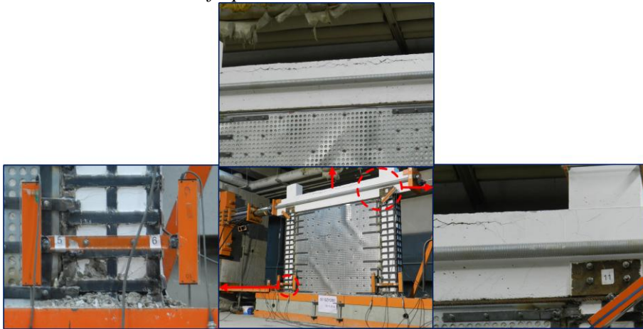
Figure 10. Failure Mode of Specimen S1ZY200
