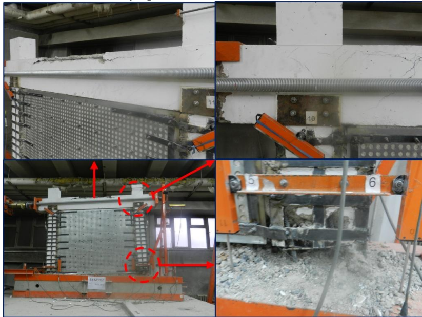
Figure 16. Failure Mode of Specimen S2ZN200
