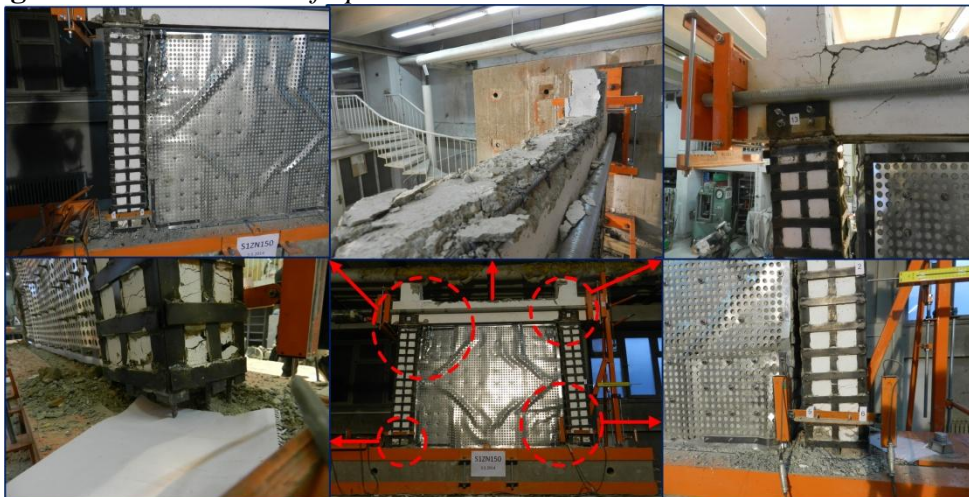
Figure 9. Failure Mode of Specimen S1ZN150
