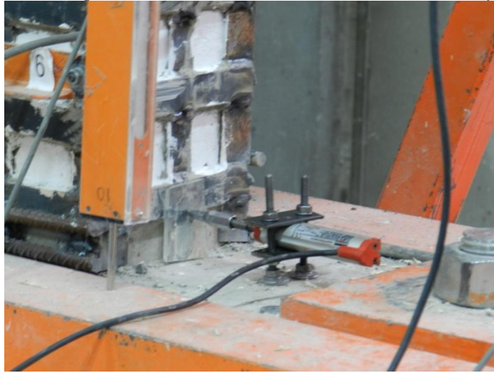
Figure 4. Lateral Displacement Measurement at the Lower End of the Column
