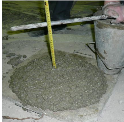
Figure 3. Measuring Slump Flow of HPC Mixtures
