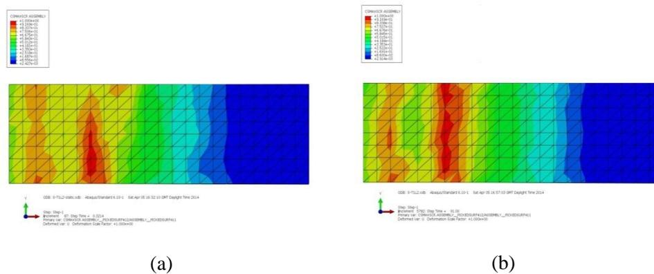
According to The legend; the red colour shows that the maximum nominal stress criterion has been satisfied and transfer of stress among CFRP and concrete has started to gradually reduce until debonding occurs, whereas the blue colour shows that the CFRP sheet is still bonded to the tension side of concrete slab. It is clear that the damaged region for both slabs (S-T1L1 & S-T1L2) is corresponding to the area of the maximum tensile plastic strain in the concrete substrate.
