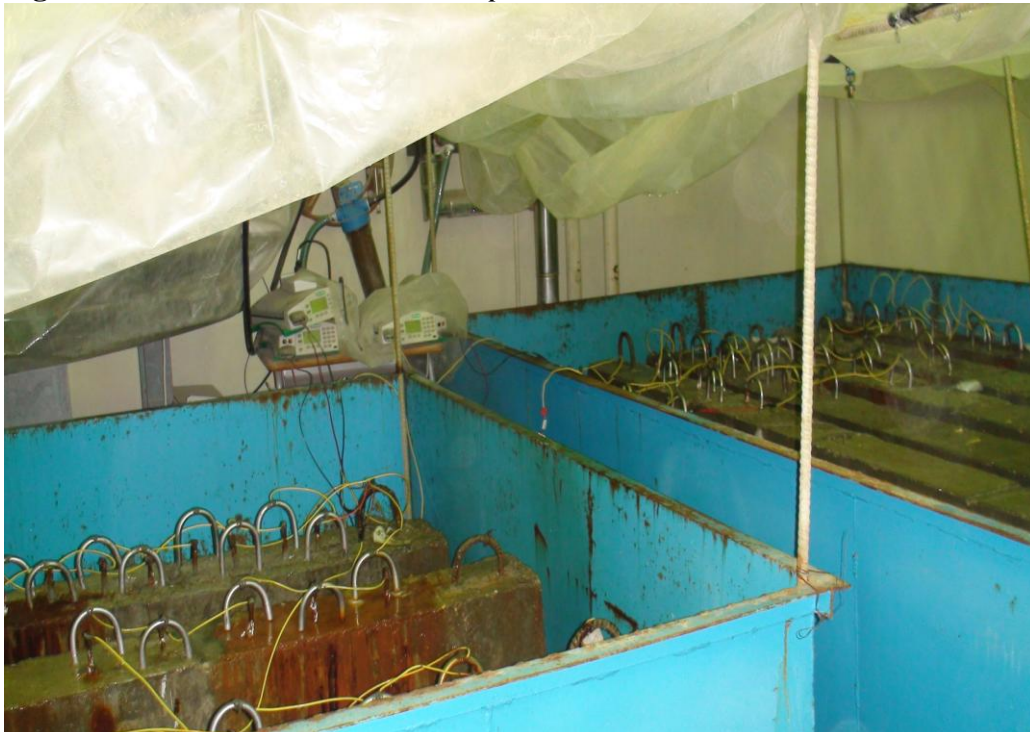
Figure 4. Accelerated Corrosion Setup
