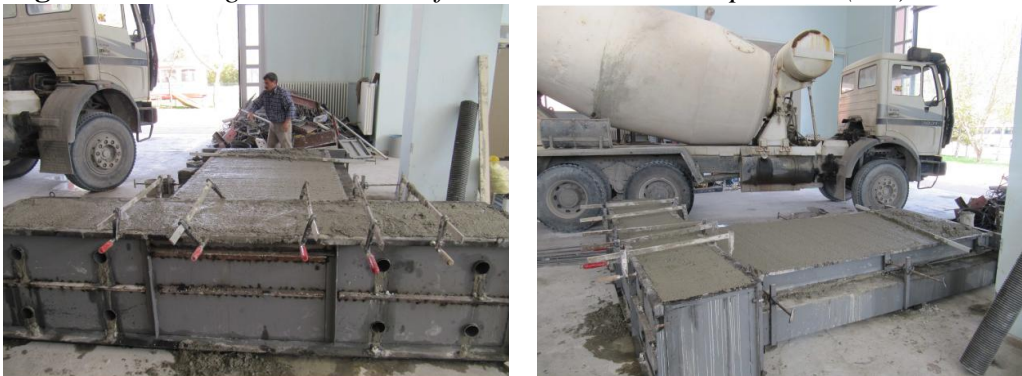
Figure 5. Pouring the Concrete of the Shear Wall Test Specimen (SW)
