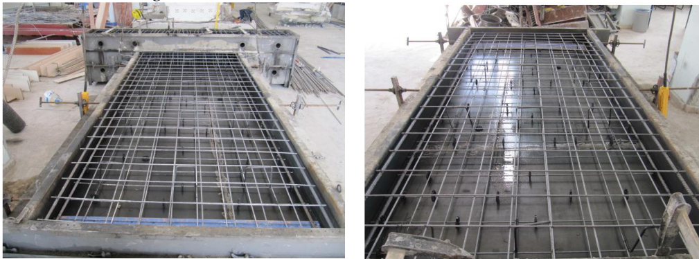
Figure 5. Pouring the Concrete of the Shear Wall Test Specimen (SW)
