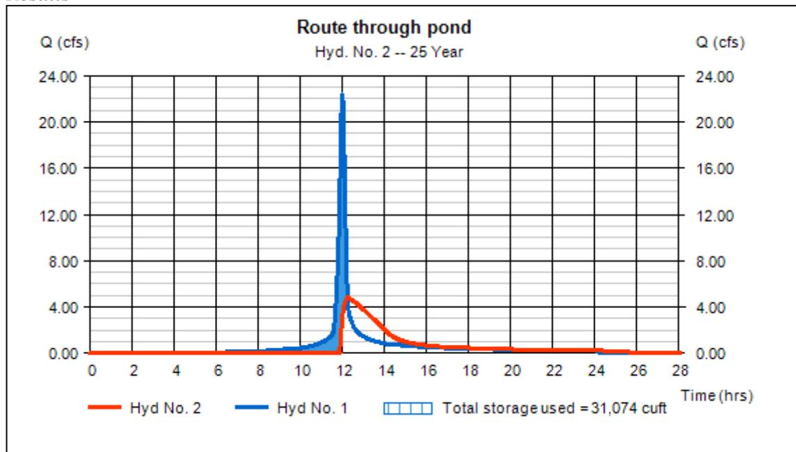
The peak of the inflow hydrograph is 22.37 ft<sup>3</sup>/s and the outflow hydrograph peak is 4.82 ft<sup>3</sup>/s. Stormwater first begins discharging from the pond at 11.83 hour at the rate of 0.007 ft<sup>3</sup>/s. At the 28 hour mark stormwater is still discharging from the pond at the rate of 0.03 ft<sup>3</sup>/s. The significance of this pond design is that it retains all first flush volume and the balance of the inflow
