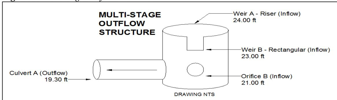
**Table 3. Multi-Stage Outflow Structure Invert Elevations**
