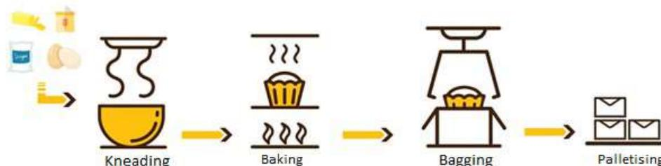
Various raw ingredients are mixed and kneaded to form a dough which is baked in an oven. Once cooked, the pastries are bagged and palletised. Several factors are involved in the completion of each task and any variation in one of them impacts the rest of the process. For example, a stoppage during baking will result in under or overcooking of pastries and their subsequent disposal. This in turn will have an impact on the number of products to be bagged and palletised.
