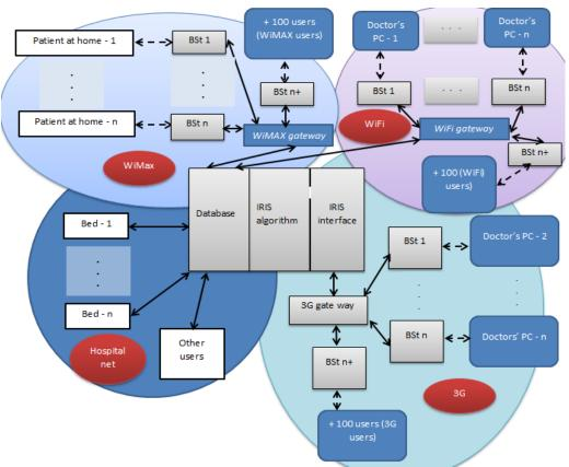
Figure 1: Diagram of Wireless IRIS network
