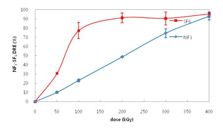
Figure 1. DREs of NF3 and SF6 gases as a function of doses.
