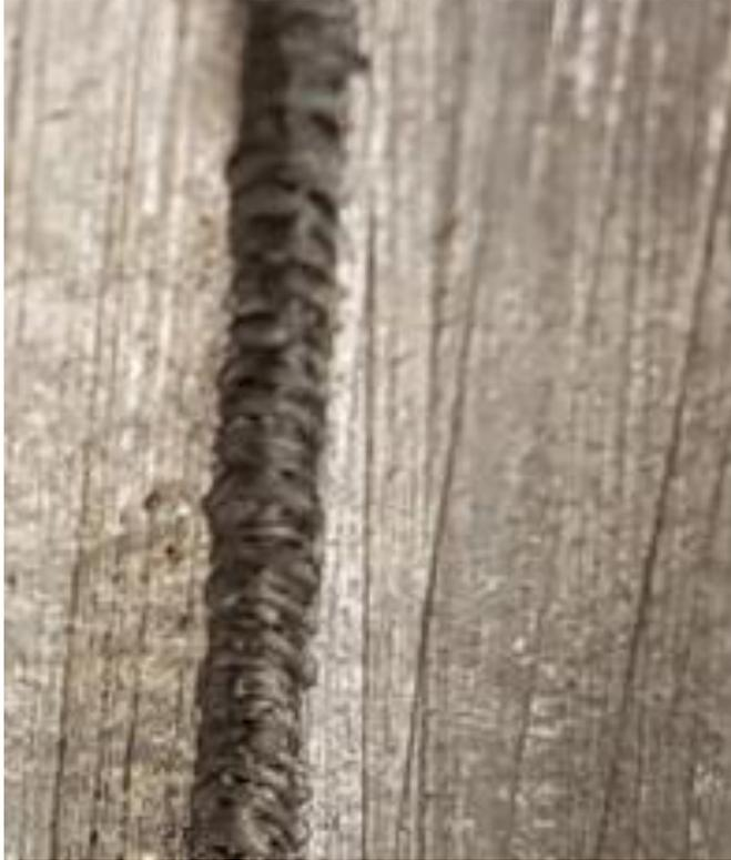
**Figure 13.** *Electron Beam Welded Joint, AM 60, No Filler Material, Cross-section View*
