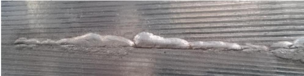
Another question deals with the type of inert gas. Every inert gas or inert gas mixture has different properties. For example, helium and argon are both inert gases, yet they do not react with the weld in the same way. Helium expands the penetration.
