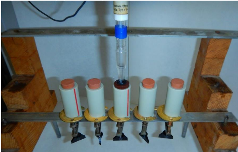
Figure 3. Configuration of the Corrosion Cells
