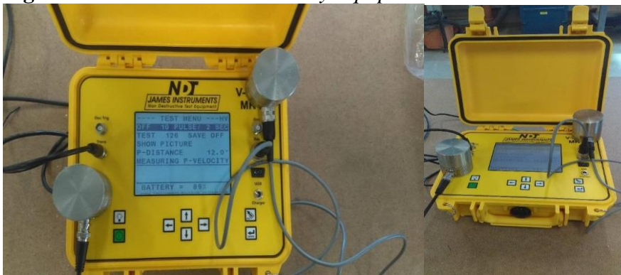
Figure 3. Ultrasonic Pulse Velocity Equipment
