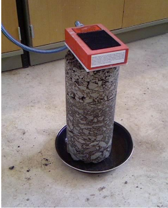
Figure 3. GPR Data Collection from an Asphalt Core Sample (Showing GPR Antenna on Top of Core and Metal Plate at Base of Core)
