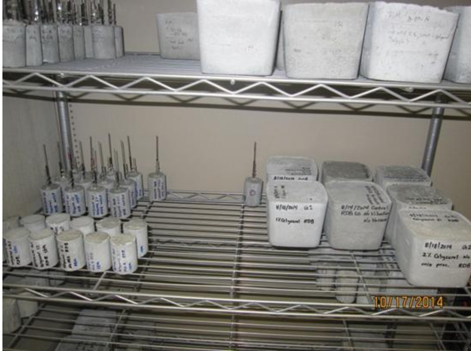
Figure 2. The Concrete Specimens in the Home-made Humidifying Chamber Stored for Curing for 28 Days. After Curing the Samples were Immersed into 3.5% NaCl Solution for Chloride Sorption. When Sufficient Time (about 560 Days) of Sorption has Passed Concrete Blocks were Drilled for Sample Collection and Chloride Analysis with Depth
