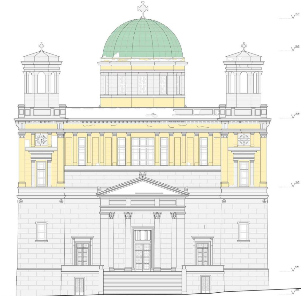
Figure 2. Main Façade Prospect (Colour Label for Materials: Grey = Marble, Yellow = Stuccoes and Plaster, Green = Copper)
