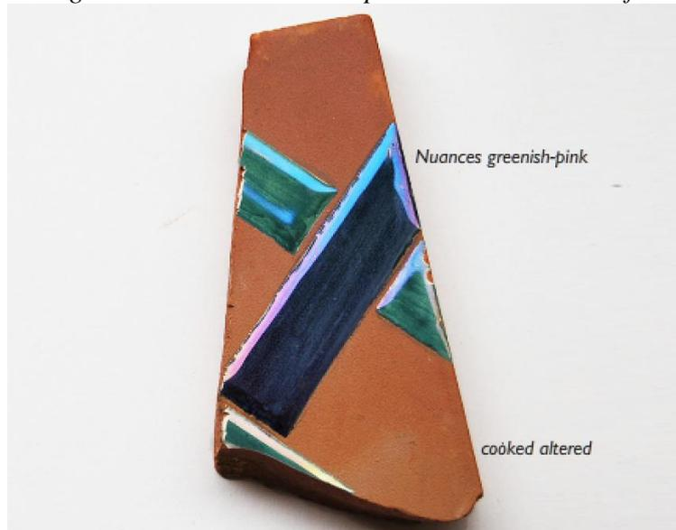
Deposition SiO<sub>2</sub> (silicon dioxide RI 1.46) by ION PLATING THERMAL PLASMA ASSISTED from source, (Figure 7, Table 1), (reactive bank), with evaporation of SiO<sub>2</sub>. Result: thin protective film, transparent, achromatic, abrasion resistant.
