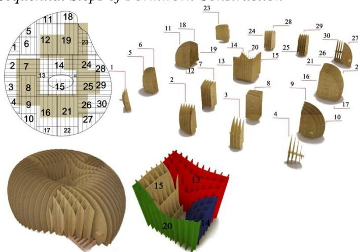
**Figure 18.** *The Process of Final Fabrication*
