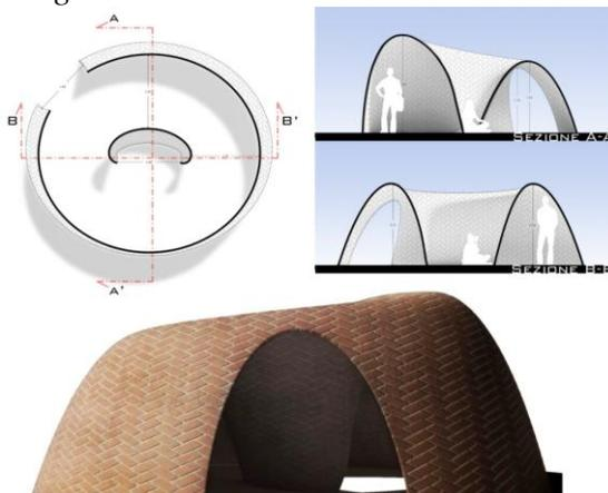
**Figure 15.** *The steps of catenary form construction*
