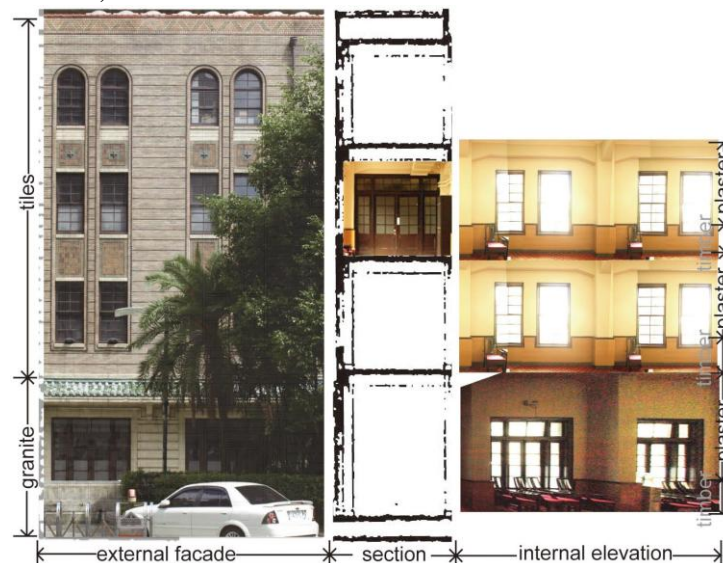
Figure 1. Diagram of the claddings of the partly southern elevation, the section with horizontal circulations and the opposite internal elevation of the Taipei Public Hall, Taiwan
