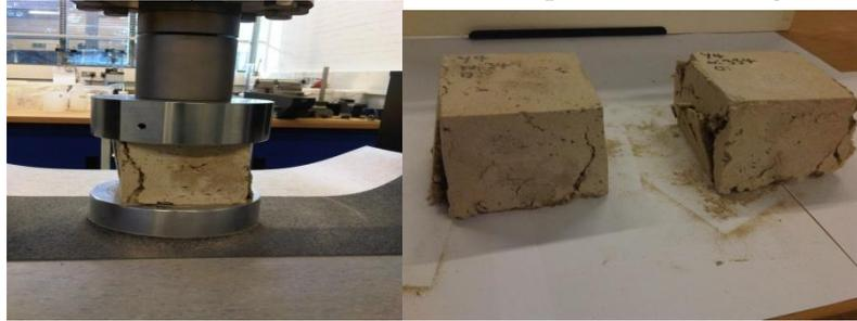
Considering that these developed lightweight materials, as other existing hempcretes, are intended to be used in combination with structural elements, such observed ductile behaviour may be attractive as it enhances the accommodation and adjustment between structural and non-structural elements which helps improve the absorption of small displacements and dumping, which always occur in houses and buildings [13].
